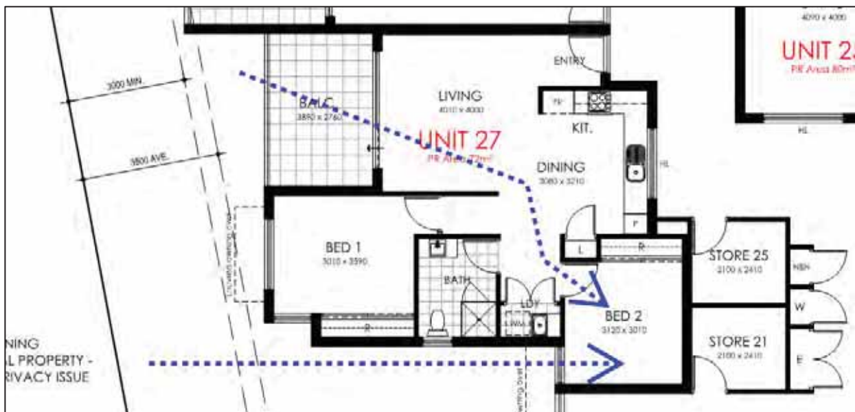
Figure 1 - Natural Ventilation to Bedroom 2 of Apartments 13, 20 and 27
